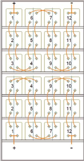
In general, connect the batteries using the shortest possible cables. Normally, cells are connected in series with alternating polarity, resulting in the shortest possible connector length.
