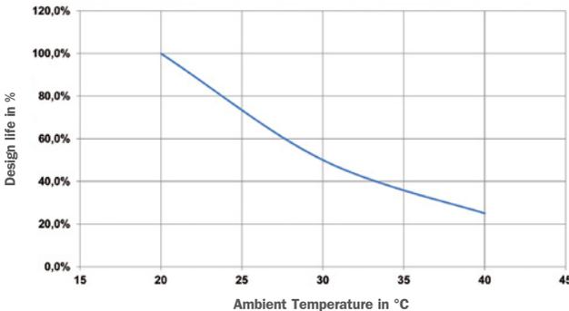
Fig. 7-7: Design life of un | power vRL (OPzV solar.power) cell as a function of ambient temperature (standby application in float charge operation with 2.25 V/cell)
